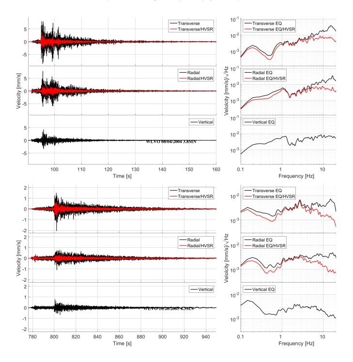
Figure 7: WLVO earthquake record (left) and spectra (right) for both considered earthquakes. (Black) original earthquake waveform and spectra, (Red) Waveforms and spectra of horizontal components corrected by HVSR model
