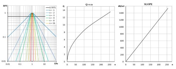
Figure 3: (left) Filter response for normalized f; (middle and right) Quality factor and Slope as a function of slope steepness(n) Equations (4 and 6)
