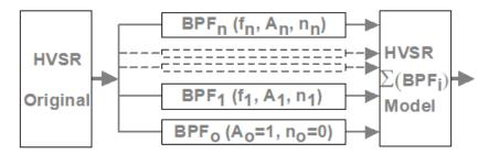
Figure 4: Simplified procedure for estimating a parametric HVSR spectral model
